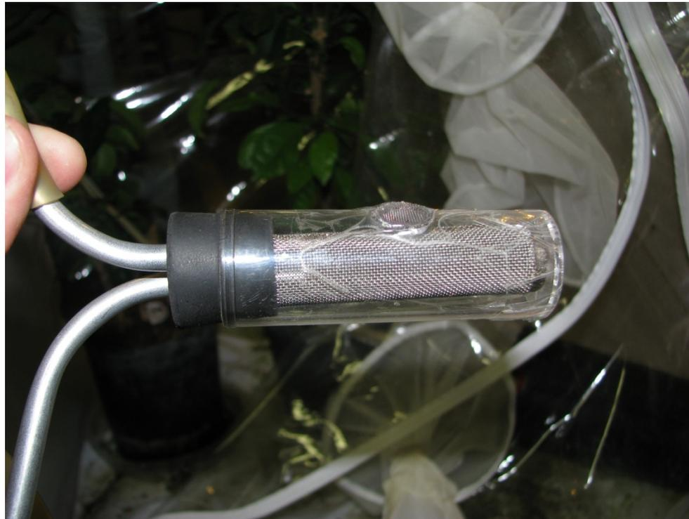
Figure 1. Method of collecting adult Asian citrus psyllid (ACP), *Diaphorina citri*, into 30-mesh stainless-steel cages using a standard mouth aspirator apparatus.
