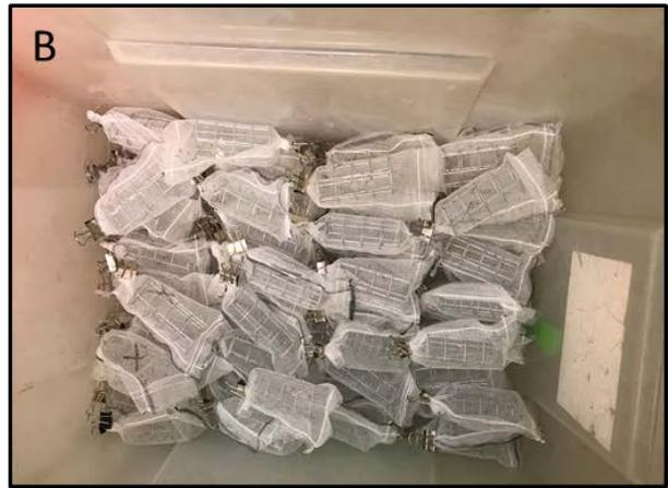
Figure 2. Nylon mesh cages containing fiberglass filter paper (A) and containing ACP (B). Note that the open end of the nylon cage was closed using a binder clip.
